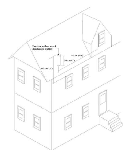
□ The exterior pipe termination of the passive stack terminated above the roof top shall be directed vertically in accordance with the following:
